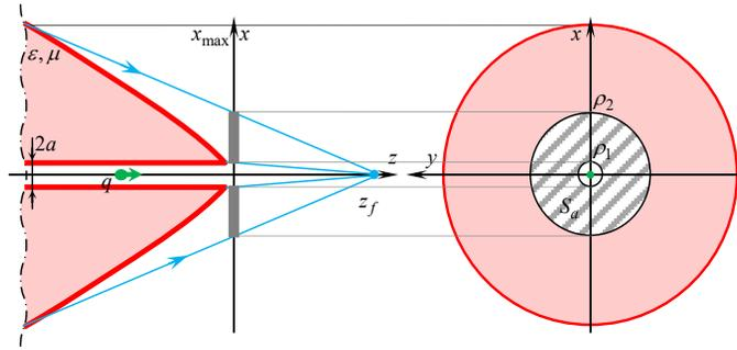
Figure 2: Ring aperture  $S_a$  for Stratton-Chu formulas.
