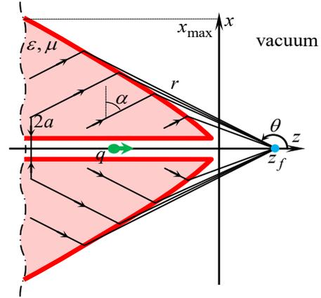
Figure 1: Geometry of concentrator ( $x-z$  cut).
