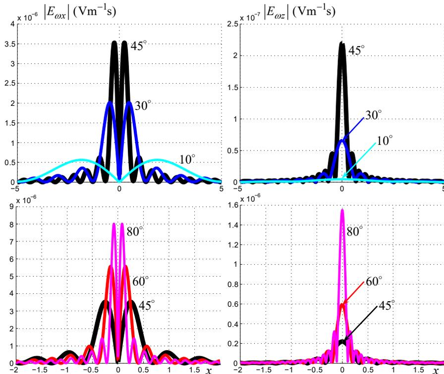
Figure 4: Transversal (left column) and longitudinal (right column) components of the electric field over line parallel to  $x$ -axis for  $z = z_f = 5\text{ cm}$ ,  $f = 5\text{ cm}$ ,  $\beta = 0.8$ ,  $\omega = 2\pi \cdot 1\text{ THz}$ ,  $x_{\text{max}} = 10\text{ cm}$ . Number near curve indicates  $\alpha$ .
