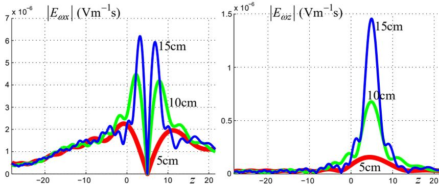
Figure 3: Behaviour of the transversal ( $E_{\omega x}$ ) and longitudinal ( $E_{\omega z}$ ) components of the electric field over the ray with  $\theta = 178.5^\circ$ . Other parameters are:  $z_f = 5\text{ cm}$ ,  $f = 5\text{ cm}$ ,  $\beta = 0.8$ ,  $\varepsilon = 2$ ,  $\omega = 2\pi \cdot 1\text{ THz}$ . Number near curves indicates transversal target size  $x_{\text{max}}$ .
