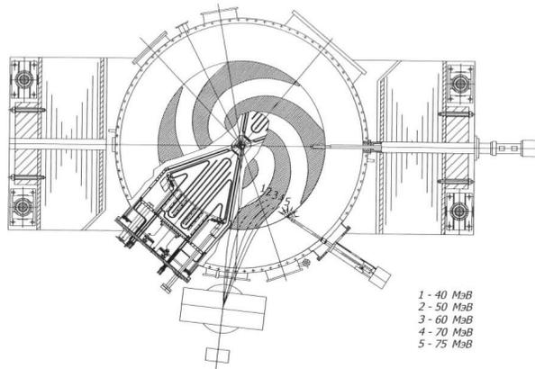
Figure 3: Schematic view of the extraction system of C-80 cyclotron.
