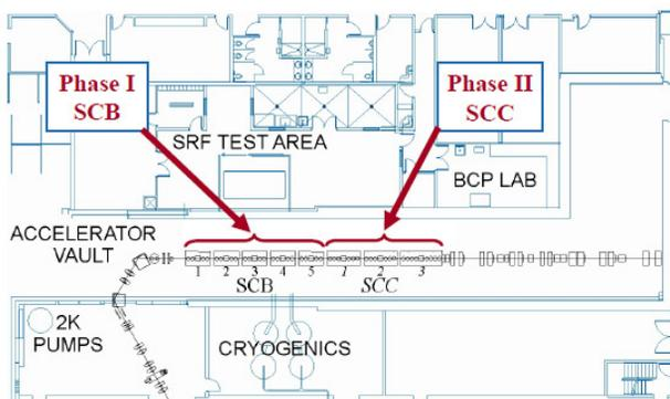
Figure 1: Layout of ISAC-II linac and SRF infrastructure.
