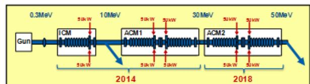
Figure 3: The stages of the eLinac project.
