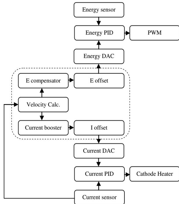
Figure 5: Schematic diagram of stabilization systems.
