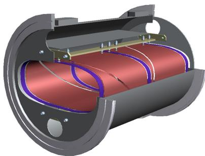
Figure 1: A large (400 mm) aperture, super-elliptical, split plate BPM design in dispersive section provides a larger linear response aperture.
