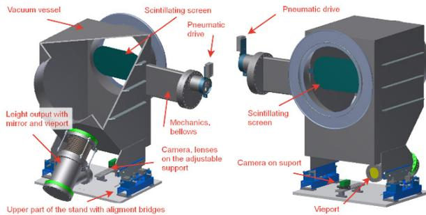
Figure 4: Scintillating screen and its cross section.
