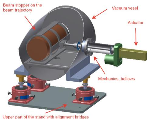
Figure 5: Faraday cup with longitudinally sectioned body.
