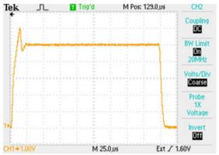
Figure 4: The waveform of the valve power supply output current. The vertical scale is 10 A/div, horizontal scale  $-25 \mu s/div$ .
