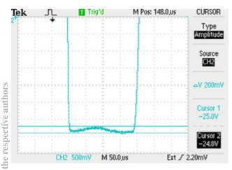
Fig. 6. Waveform of the output pulse top of extraction voltage power supply. Vertical scale - 500 V/div, horizontal scale -  $50 \mu \text{S/div}$ .
