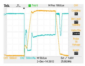
Figure 3: The oscillograms of voltage and discharge current of the H-minus ion source. The top beam (blue) is the voltage at discharge, 50 V/div. The lower beam (yellow) is the discharge current, 10 A/div. Horizontalscale - 50  $\mu$ s/div.
