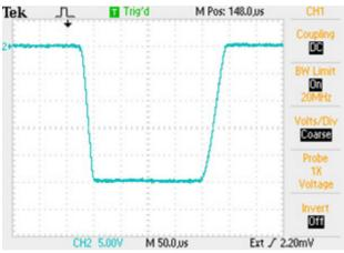
Figure 5: The waveform of the output pulse of extraction voltage power supply. Vertical scale - 5 KV/div, horizontal scale - 50  $\mu$ S/div.
