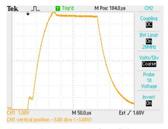
Figure 2: The output current of gas discharge power supplies. Vertical scale -20 A/div, horizontal scale -50  $\mu$ s/div.
