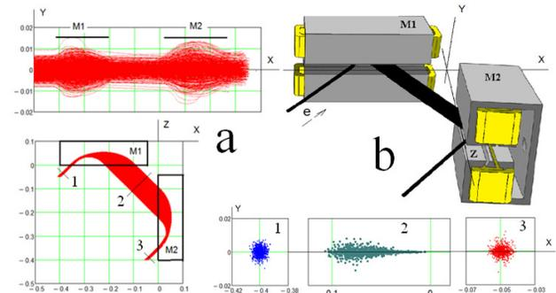
Figure 4: Calculation of beam bending on 180°.
