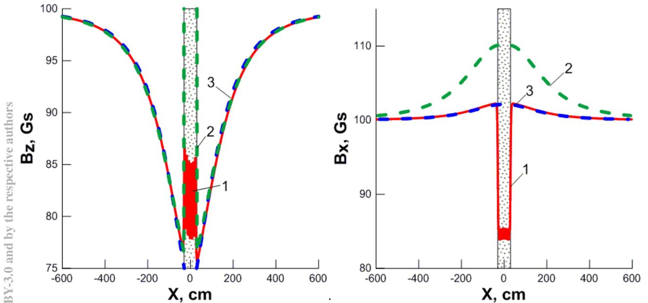
Figure 2: 100 Gs field disturbed by reinforced concrete structure. Field co-planar ( $B_z$ ) or normal ( $B_x$ ) to rebar. 1 – detailed models, 2 – homogeneous isotropic models, 3 – single-layer models.
