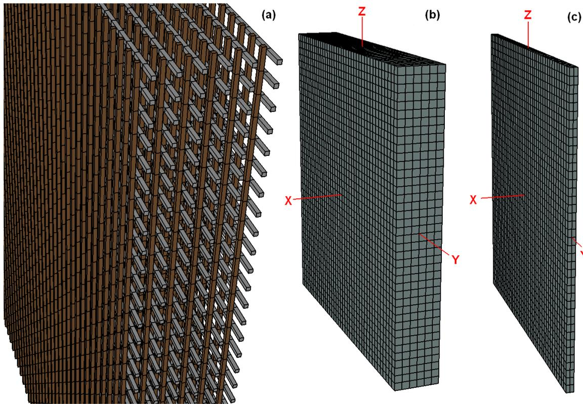
Figure 1: Computational models for test problem with a set of criss-cross rebar layer magnetized in parallel or perpendicular to layers external field: detailed (a), homogeneous isotropic (b) and single-layer (c) models, prepared for KLONDIKE code [8].
