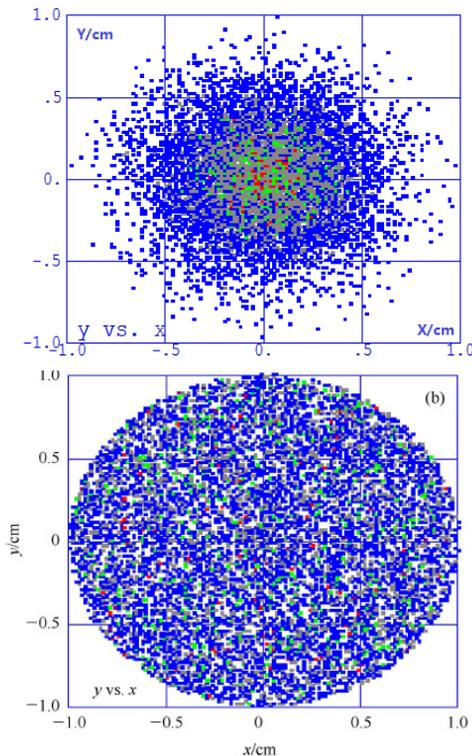
Figure 2: The electrons' Gaussian and Uniform distributions.
