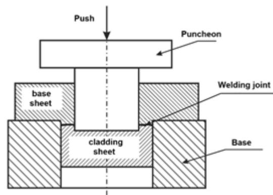
Figure 6: The scheme of layer tear test.
