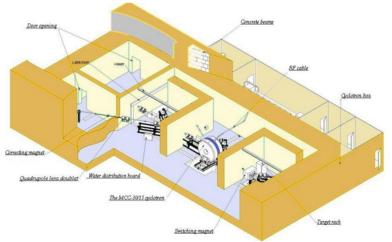
Figure 5: One of possible layouts of the cyclotron system.
