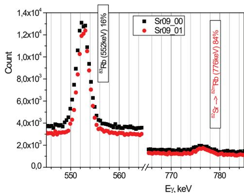
Figure 2: Gamma spectrum of RbCl before heating.
