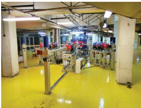
Figure 1: Cyclotron C-80 (ground floor) with three proton beam lines to the target stations (cellar).
