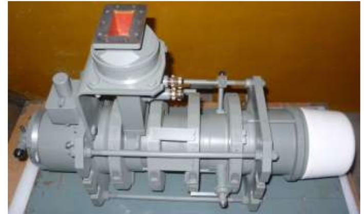
Figure 2: Klystron KIU-168, pulsed power 3.5 MW.
