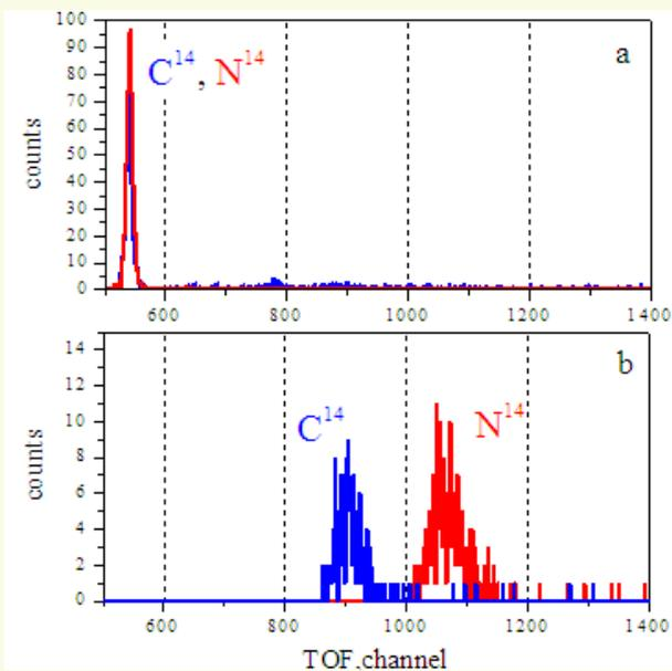
The time-of-flight of ions at the exit of AMS (a) and same, but after passing through 2.5um Mylar film (b).
