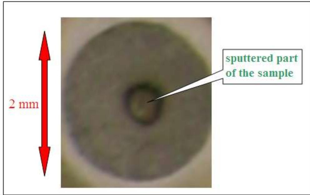
The sample in the ion source sputtered by cesium beam.
