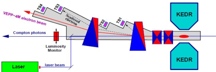
Electron tagging system for two-photon experiments
