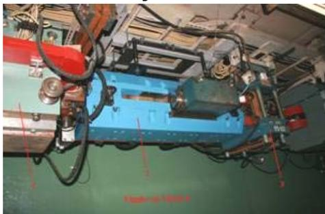
7-pole electromagnet wiggler Installed recently at VEPP-4M
