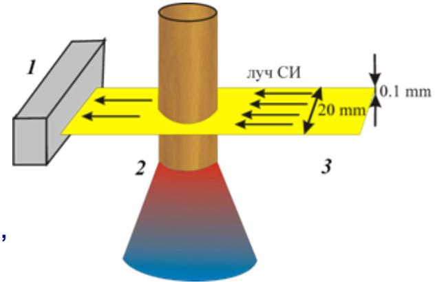
Experimental setup for density distribution reconstruction.
