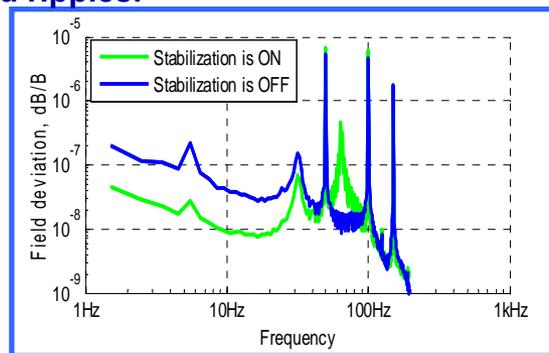
The graph shows that at a frequency of 5 Hz suppression of ripples is more than by 10 times, at a frequency of 10 Hz - 3 times, at a frequency of 30 Hz - 2 times.
