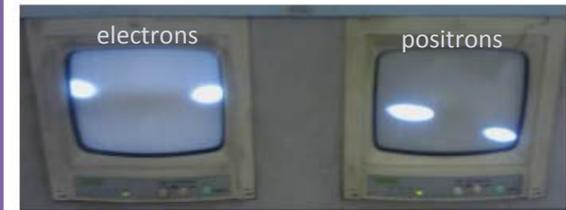
Figure 6: SR images of the 1.1 mA electron (left) and the 0.3 mA positron (right) bunches on the TV monitors while applying the RF separation at the 6.5 kV peak voltage. Electrostatic separation system is fully off.
