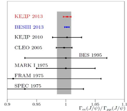
The ratio of the electron and muon widths of the  $J/\psi$  meson has been measured using direct  $J/\psi$  decays. The measurement result  $\Gamma_{e+e} / \Gamma_{\mu+\mu}$  is in a good agreement with the lepton universality
