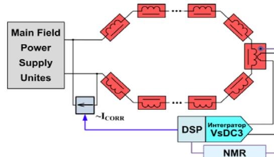
The essence of the method is measuring the field ripples by the induction sensor to adjust the current in the magnet with the help of parallel connected to IST current generator, which is opposite to the measured ripples.
