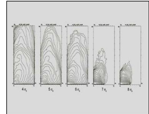
Distribution in plane of betatron amplitudes at various values of orbit separation in TS
