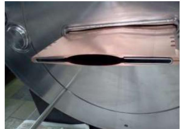
Copper liner for the high field wigglers
