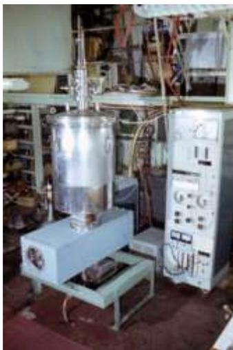
*The first superconducting 20-pole wiggler (“snake”), assembled with cryostat, before installation on the ring (1979)*
