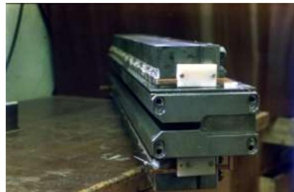
*The magnet system of the first superconducting 20-pole wiggler (“snake”) (1979)*
