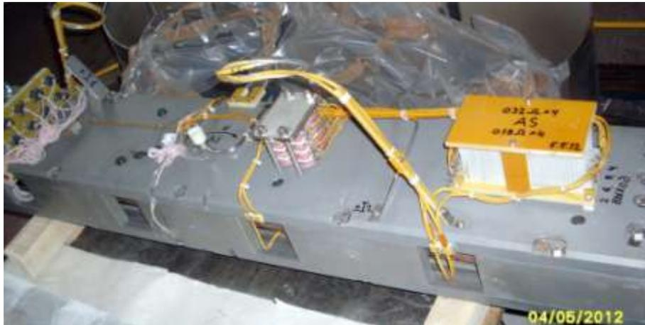
Quench protection system with cold diodes and dump resistors
