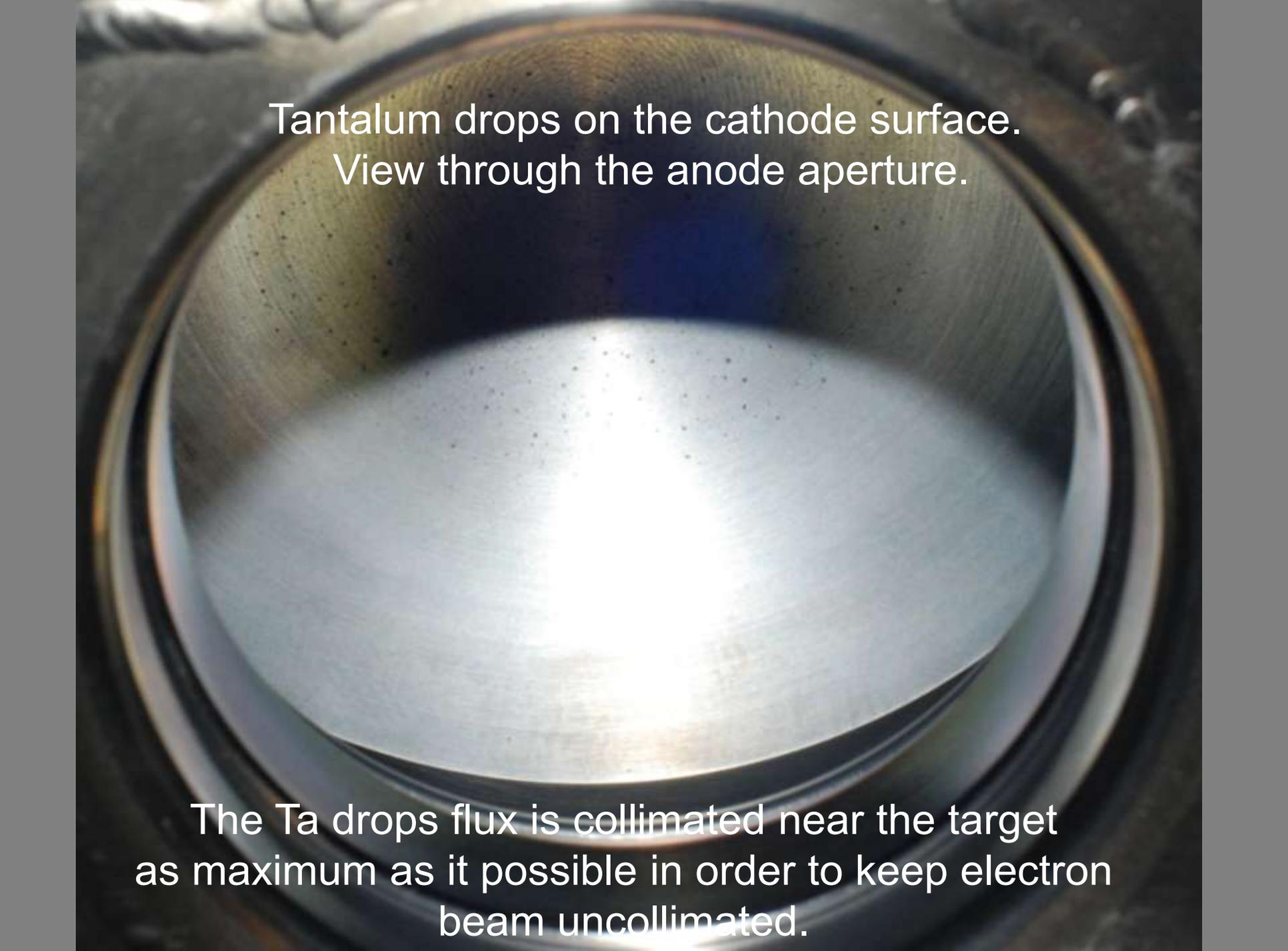
A close-up photograph looking through a circular anode aperture. The central area is a bright, circular spot of light, representing the tantalum drops flux. The surrounding area is dark, and the metal surfaces of the aperture and cathode are visible.
