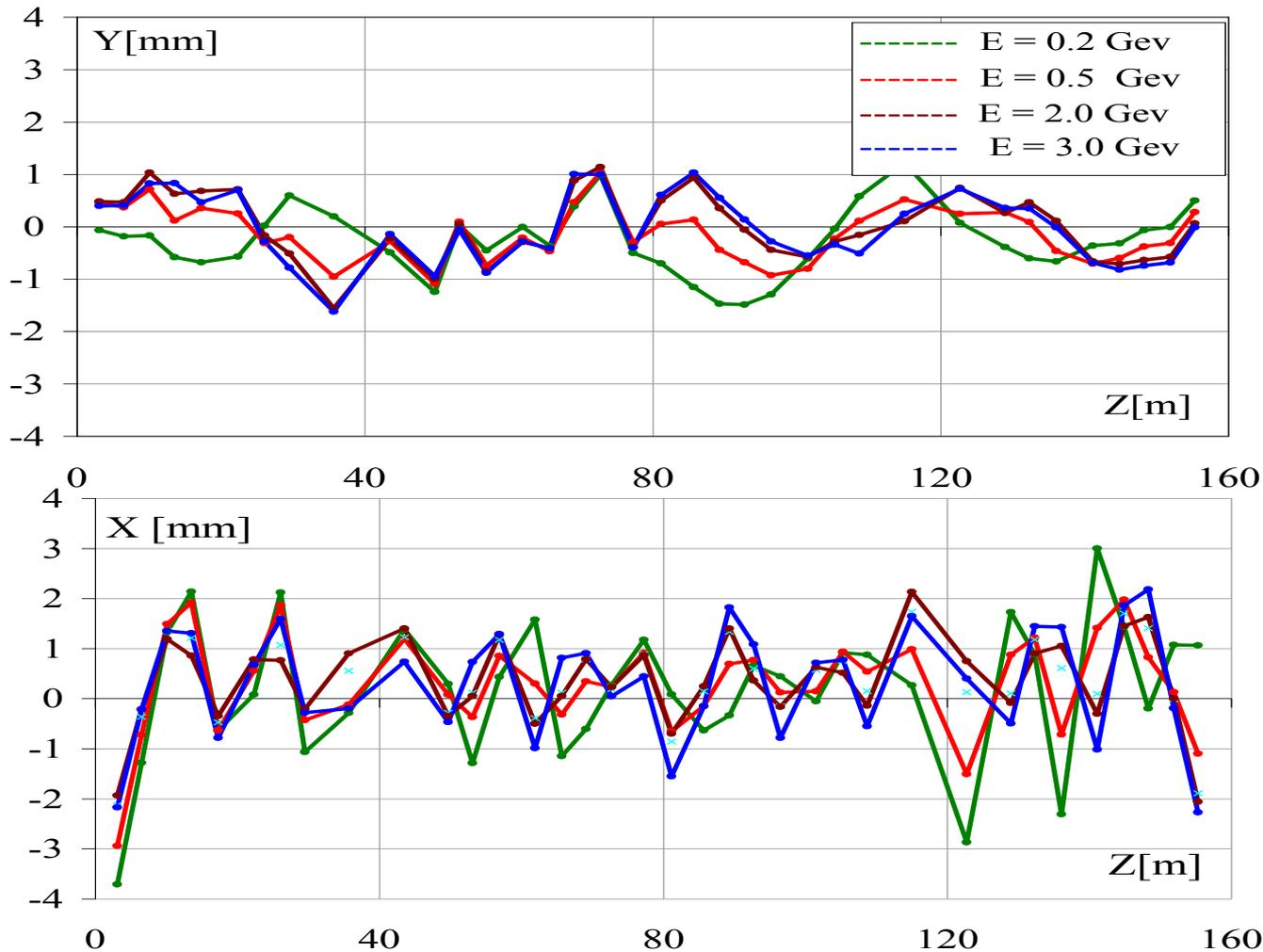
Vertical and horizontal orbit of beam along the whole ramp
