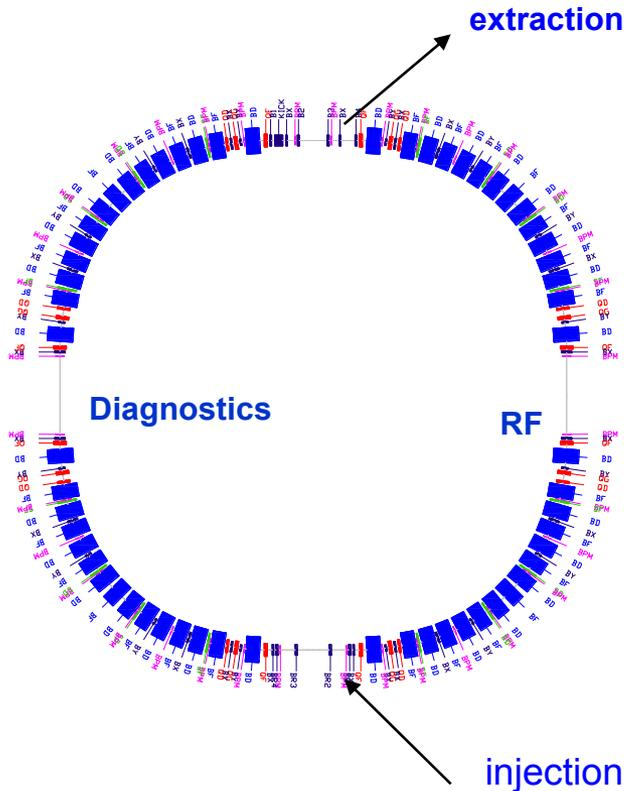
The magnetic lattice includes four quadrants. Every quadrant contains five regular cells with two modified cells at the ends of the quadrant for dispersion suppression.
