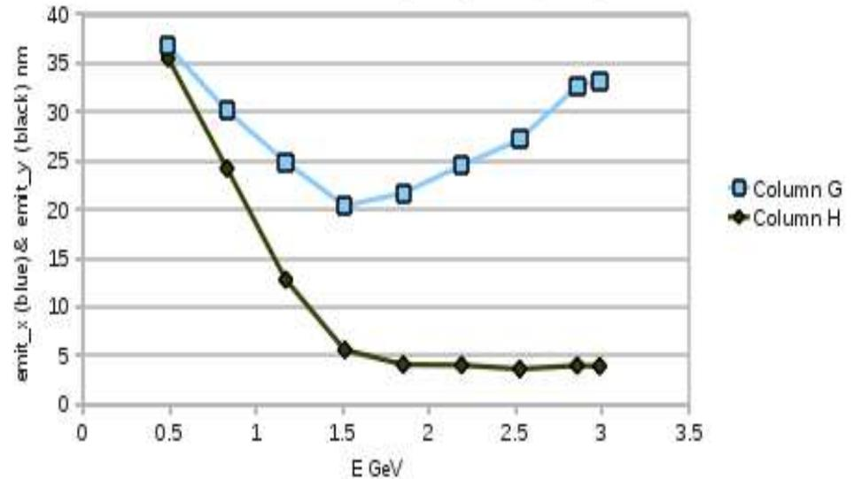
Horizontal and vertical emittance during the acceleration cycle as determined by the profile of the synchrotron light seen by the BR-A1SLM monitor
