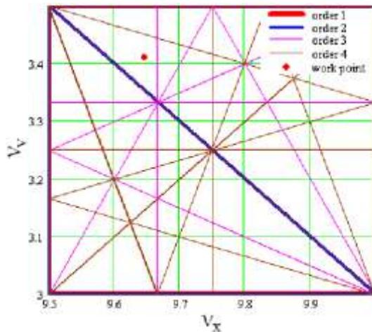
Working point at the betatron tune diagram together with resonances (up to the 4th order).
