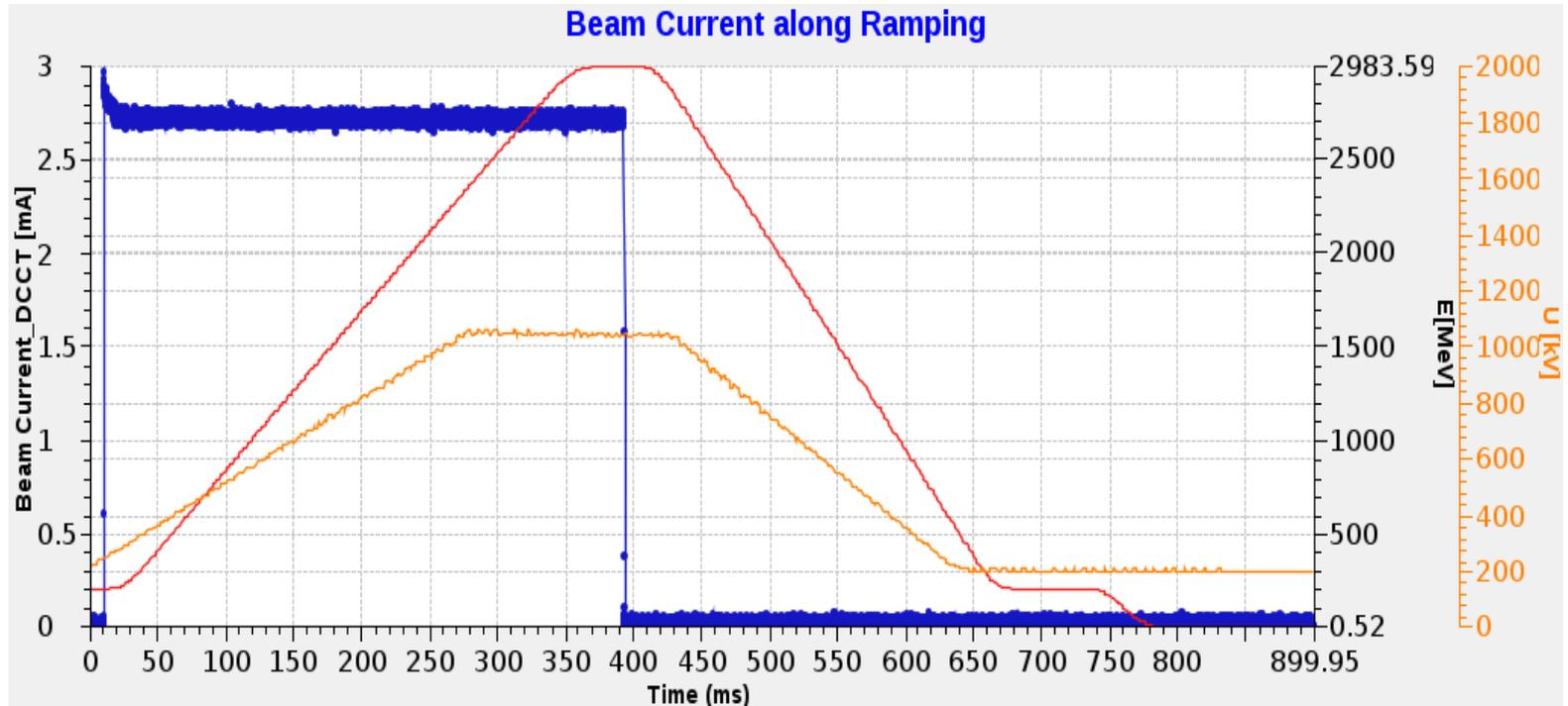
The beam current from DCCT (blue), the beam energy according dipole magnet currents (red) and the RF cavity voltage (orange) during 1Hz-cycle.
