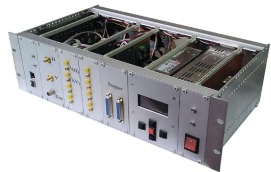
Assembled LLRF module includes two-channel signal generator, two multichannel RF vector detector modules and electronics to control the position of plungers.
