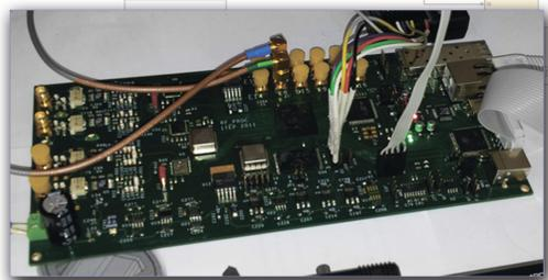
Signal generator module has onboard a pair of two-channel synthesizers, ARM microprocessor for general and remote control, FPGA for signal processing and fast interboard communication.
