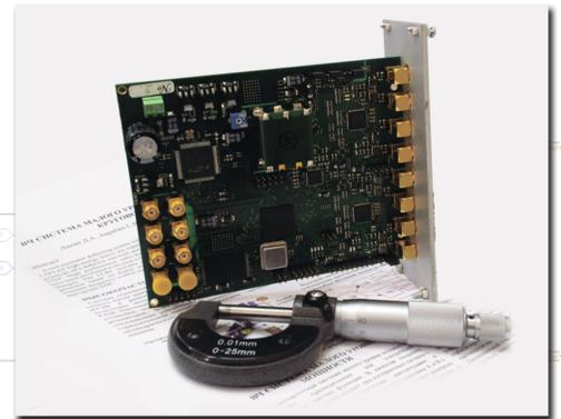
Four-channel RF signal measurement module combines on same board two ADCs with up to 100 samples per microsecond in IF mode.
