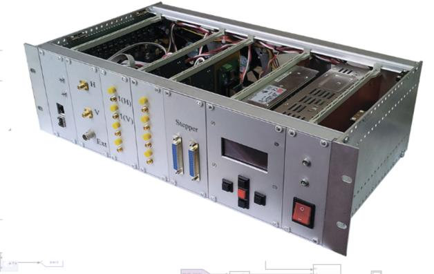
Assembled LLRF module for RF beam deflector includes two-channel signal generator, two multichannel RF vector detector modules and plunger position control electronics.
