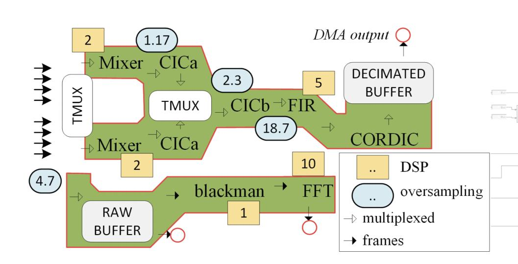
Example of an eight-channel signal processing module: the real-time branch continiously converts the ADC data stream to decimated complex ampitudes. A short-time raw data is available for postprocessing, for better performance the FFT may be executed in FPGA.
