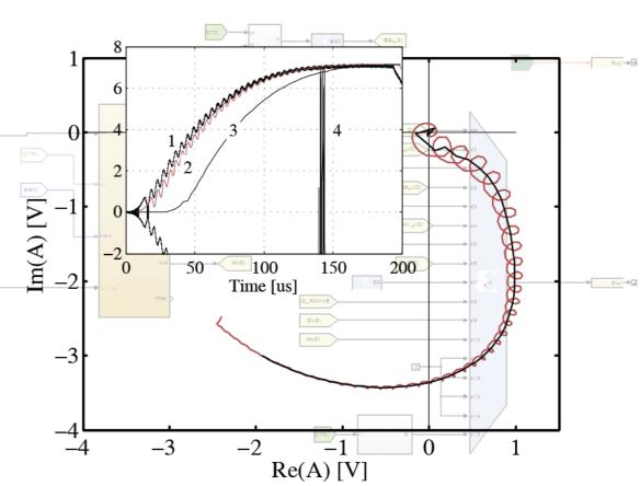
1- reference signal, 2,3-data filtered by wide/narrow band filter, 4-collecting the data for limited time extra-wideband analysis.
