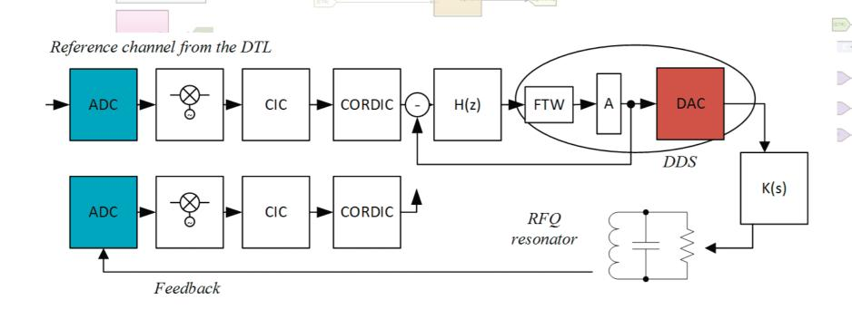
Synchronization of the novel RFQ to the existing self-exited RF system of mature drift tube linac.
