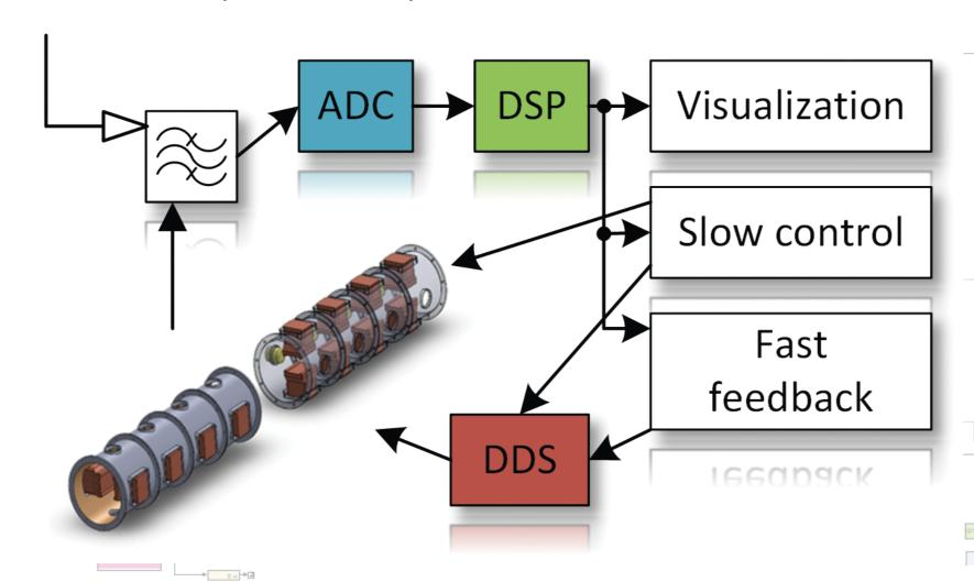
General structure of LLRF system includes generator part, measurement part and signal processor.
