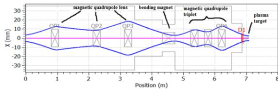
Figure 6: The beam dynamic simulation from RFQ output to plasma target.
