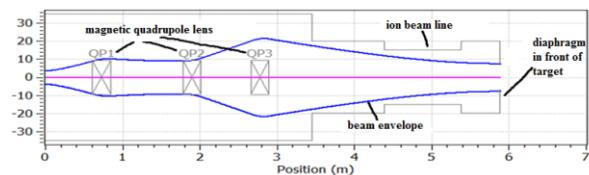
Figure 5: The beam dynamic simulation from RFQ output to target for irradiation resistance investigation of reactor construction materials with magnet ion guide
