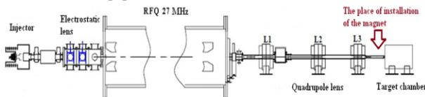
Figure 1: The Heavy Ion Prototype.
