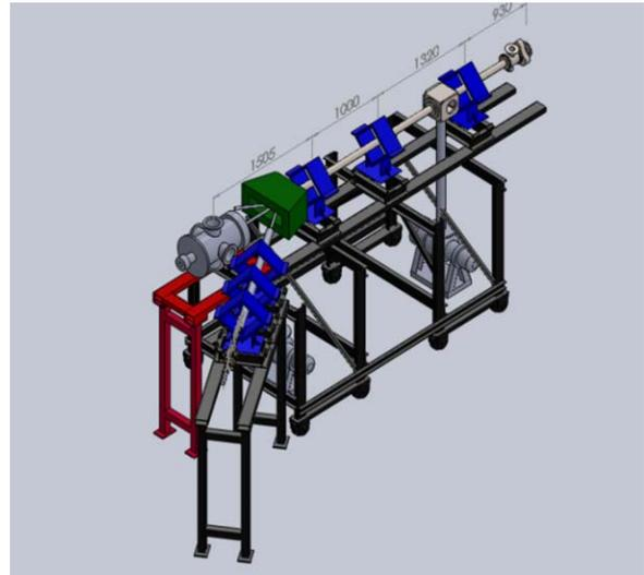
Figure 7: The general view of multifunction channel on the metal vapor target and on the plasma target at the HIP-1.
