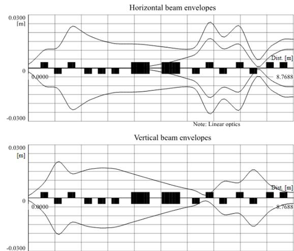
Figure 5: Beam transportation from degrader to momentum slit.
