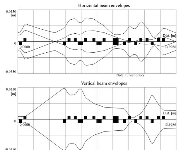
Figure 6: Beam delivery from momentum slit to entrance of treatment room.
