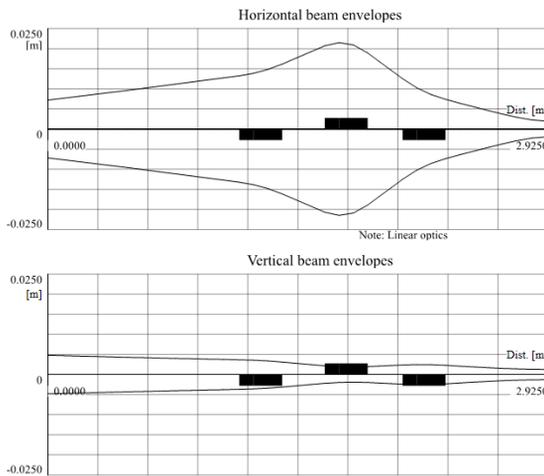
Figure 4: Beam transportation from cyclotron to degrader.
