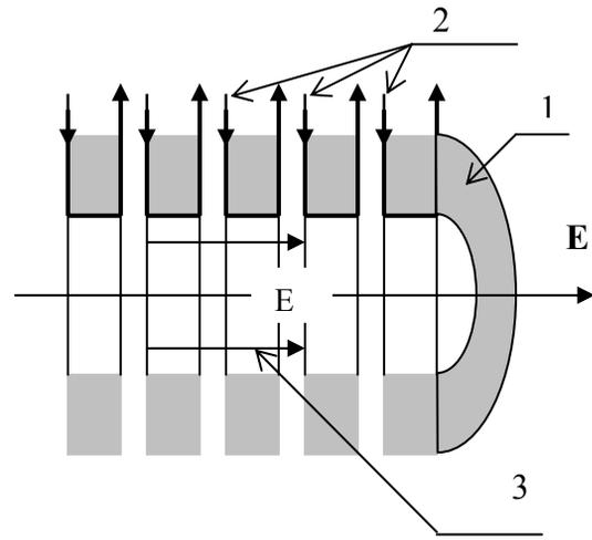
Figure 4: Schematic diagram of induction accelerating section. 1 - Ferromagnetic cores of inductors, 2 - Exciting loops of inductors, 3 - The accelerating electric field.
