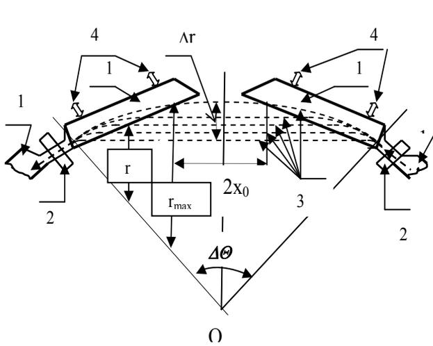
Figure 3: Special section of magnetic system. 1 - Magnetic dipoles with a uniform field, 2 - combination of quadrupole and symmetric lenses, 3 - Beam trajectories with various energy of particles, 4 - System tuning the beam trajectories.
