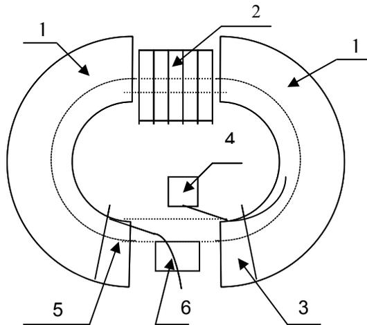
Figure 1: The scheme of the accelerator. 1 - the magnetic system with alternating focusing; 2 - the linear induction accelerating system; 3-6 - systems of input and output of electrons.
