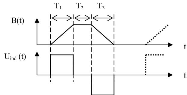
Figure 2: Diagram of magnetic induction and the accelerating pulse of induction section.  $T_1$  – Time of acceleration of electrons,  $T_2$  - Beam extraction time,  $T_3$  - Time of magnetic reversal of inductors of section.
