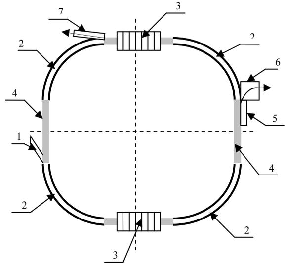
Figure 1: Scheme accelerator with a constant magnetic field. 1 - Injector; 2 - Set of special sections of magnetic dipoles; 3 - Induction accelerating sections; 4 - Straight-line segments; 5-7 - System of fast and slow beam extraction.
