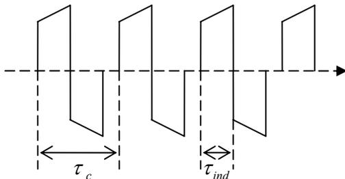
Figure 3: The accelerating induction pulses
