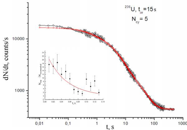
Figure 5: Time dependence of the activity of the  $^{235}\text{U}$  sample obtained in experiments №2 with irradiation time of the sample  $t_{\text{irr}} = 15$  s, presented as a count rate.
