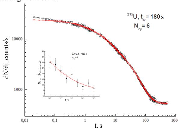
Figure 4: Time dependence of the activity of the  $^{235}\text{U}$  sample obtained in experiments №2 with irradiation time of the sample  $t_{irr} = 180$  s, presented as a count rate.
