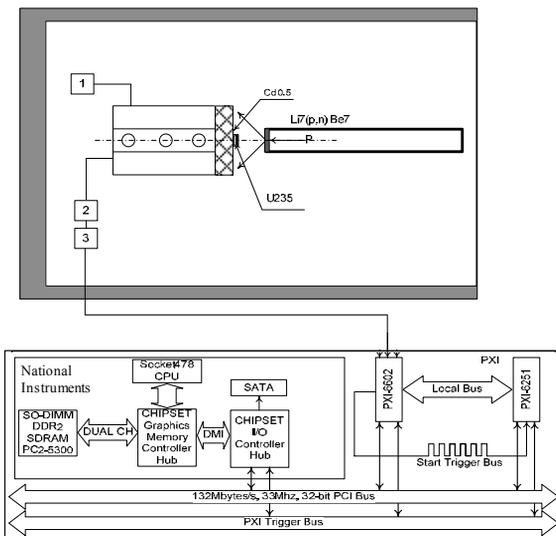
Figure 1: Block scheme of the experimental setup is performed on the basis of the system of accumulation of National Instruments. 1 – high voltage source; 2 – preamplifiers of signals from the counters SNM-18; 3 – summator of signals from the preamplifier of detector counters.
