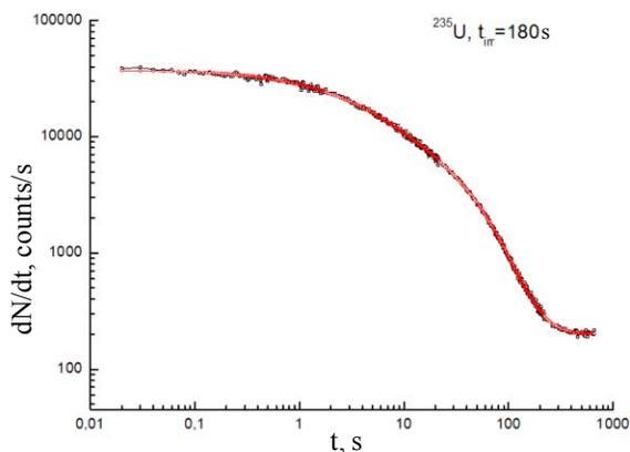
Figure 2: Time dependence of the activity of the  $^{235}\text{U}$  sample obtained in experiments №1 with irradiation time of the sample  $t_{irr} = 180$  s, presented as a count rate.
