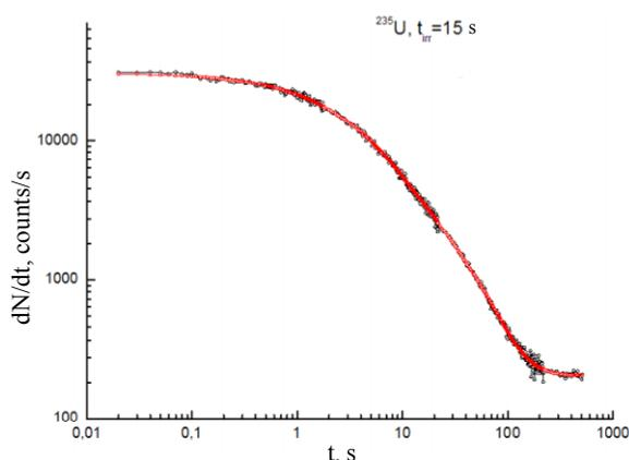
Figure 3: Time dependence of the activity of the  $^{235}\text{U}$  sample obtained in experiments №1 with irradiation time of the sample  $t_{irr} = 15$  s, presented as a count rate.
