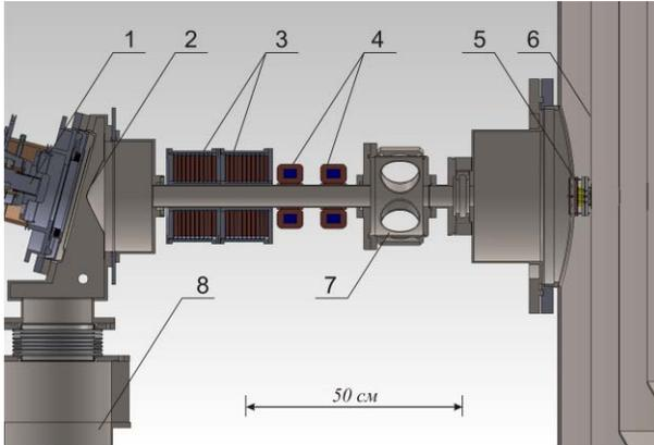
Figure 2: The scheme of existing injector: 1 –  $H^-$  ion source; 2 – cone diaphragm; 3 – focusing solenoids; 4 – magnetic beam corrector; 5 – beam aperture; 6 – first accelerator electrode; 7 – beam diagnostics; 8 – turbomolecular pump.
