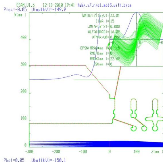
Figure 5: The ion beam transportation through the pre-acceleration tube.
