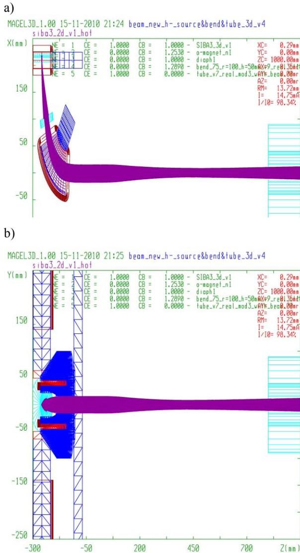
Figure 6: The ion beam transportation through the low energy beam line, 1-st stage of tandem acceleration and stripping target.
