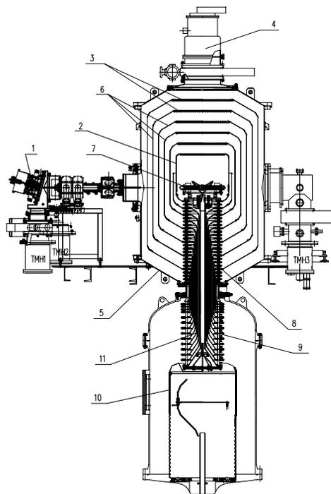
Figure 1: Scheme of the VITA facility. 1—ion source ( $H^-$ ); 2 – high voltage electrode; 3 – electrode shutters; 4 – cryo pump; 5 – accelerator vacuum volume; 6 – intermediate electrodes; 7 – stripping target; 8 – feedthrough insulator (vacuum part); 9 – feedthrough insulator (gas part); 10 – high voltage source; 11 – coaxial feeding tubes.
