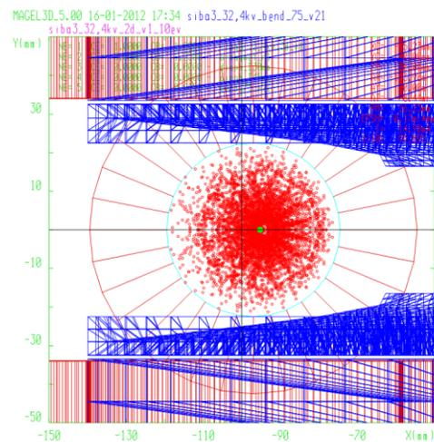
Figure 4: Beam profile at the bending magnet exit.
