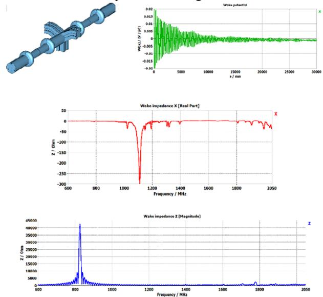
Figure 7: a). Array of 4 cells with ridged waveguide; b). Wakepotential; c). Transverse impedance; d). Longitudinal impedance.
