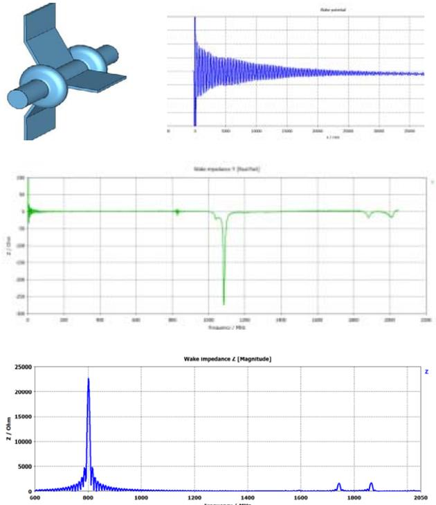
Figure 3: a). Array of 2 cells with attached waveguide; b). Wake potential; c). Transverse potential; d). Longitudinal impedance.
