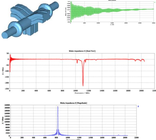
Figure 5: a). Array of 2 cells with ridged waveguides; b). Wake potential; c). Transverse potential; d). Longitudinal impedance.
