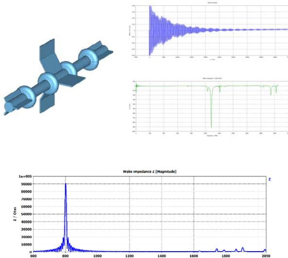
Figure 6: a). Array of 4 cells with waveguides; b). Wake potential; c). Transverse impedance; d). Longitudinal impedance.
