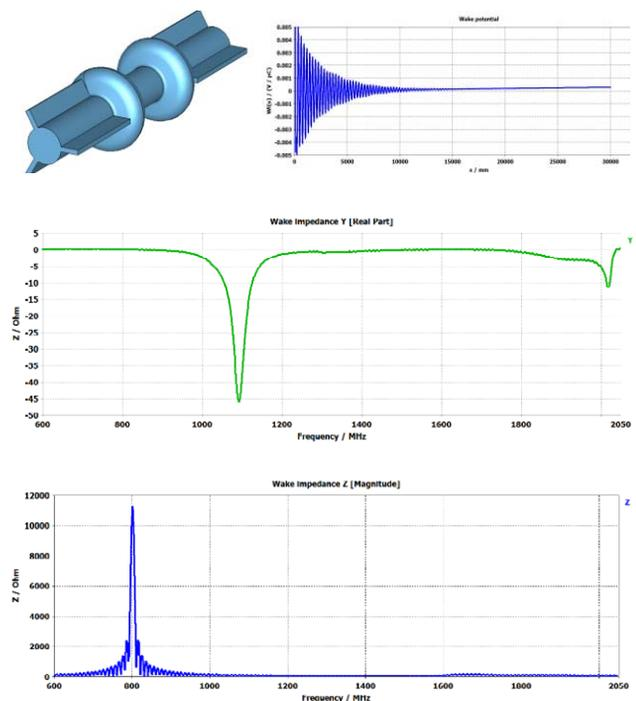
Figure 1: a). Array of 2 cells with fluted beam pipe; b). Dipole wakefield; c). Transverse impedance; d). Longitudinal impedance.
