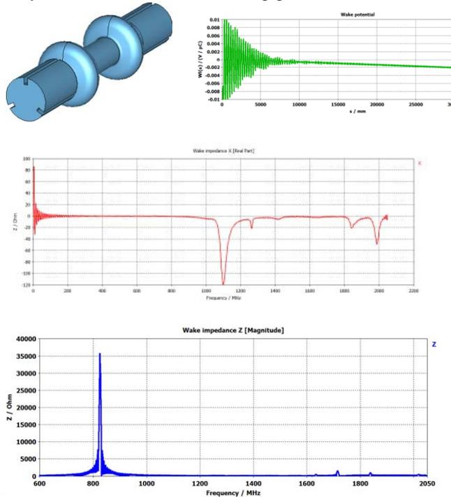
Figure 2: a). Array of 2 cells with ridged beam pipe; b). Wake potential; c). Transverse impedance; d). Longitudinal impedance.
