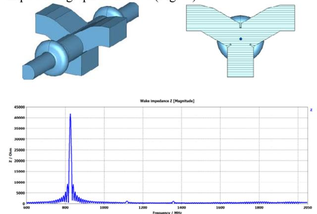
Figure 4: Array of 2 cells with attached wide waveguide and Longitudinal impedance.
