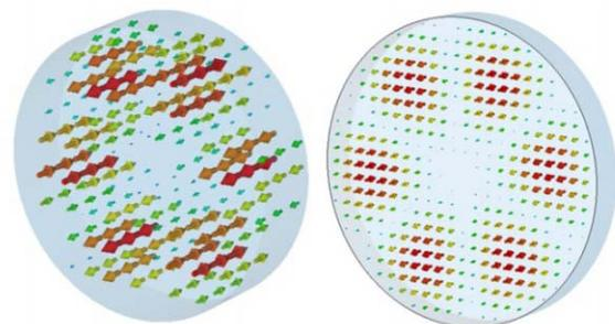
Figure 4:  $E_{310}$  field lines in the pillbox cavity.
