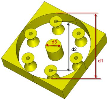
Figure 6: The geometry with a coaxial core.
