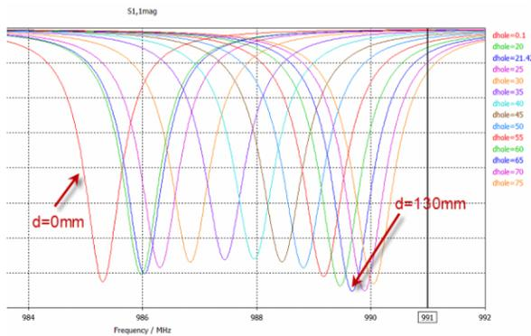
Figure 10: recess diameter variation.
