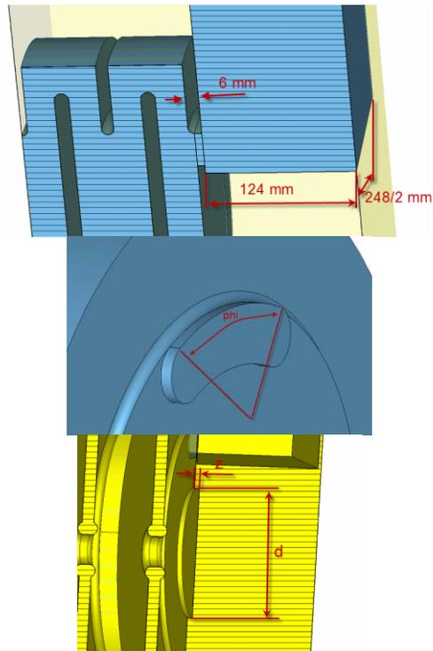
Figure 9: waveguide to accelerating structure connection.
