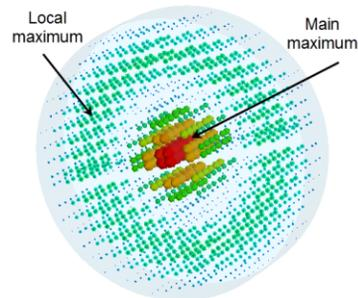
Figure 2:  $E_{020}$  mode field lines in a pillbox cavity.
