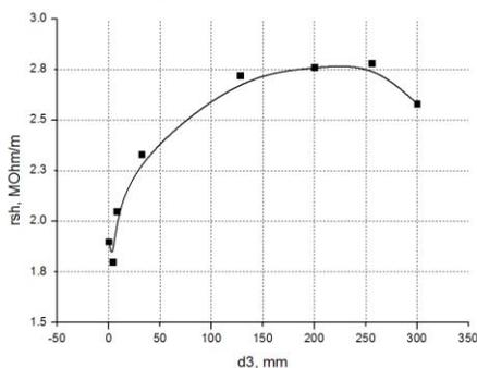
Figure 7: Rsh dependence from the core diameter.
