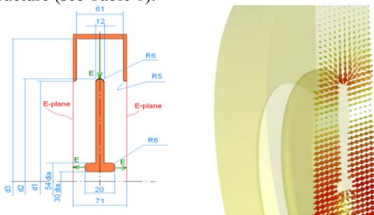
Figure 1. Accelerating structure geometry and field lines in it.
