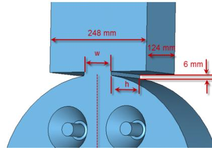
Figure 8: Waveguide to resonator connection
