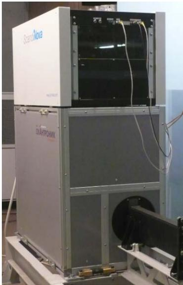
Figure 4: Accelerator for cargo inspection..
