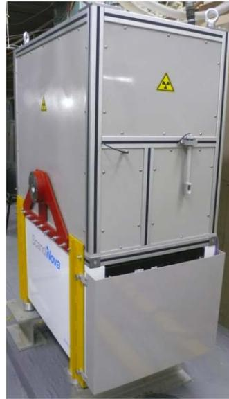
Figure 2: Accelerator for radiography.
