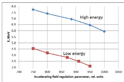
Figure 5: Low and high beam energy regulation.
