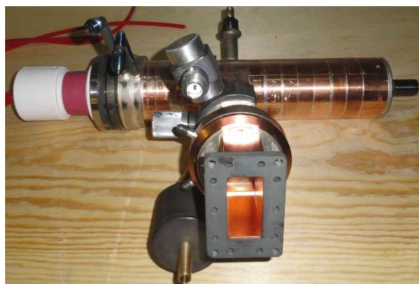
Figure 1: Accelerating system.
