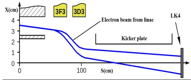
Figure 5: Scheme of angle measurement experiment.
