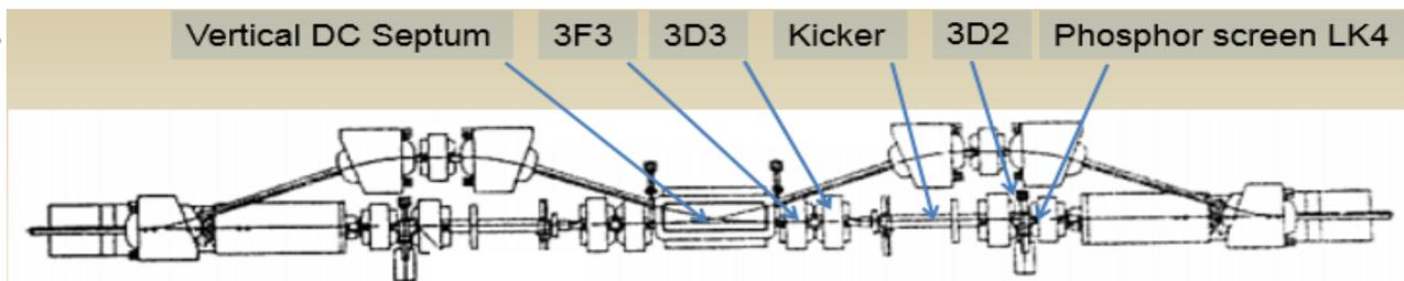
Figure 4: Injection transport line. 3F3, 3D3, 3D2 – quadruple lenses after septum magnet.
