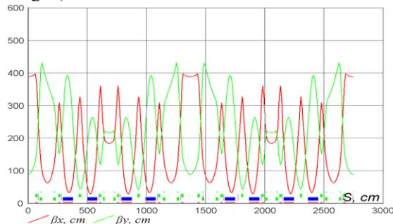
Figure 7: Beta functions for project optics in VEPP-5 dumping ring.
