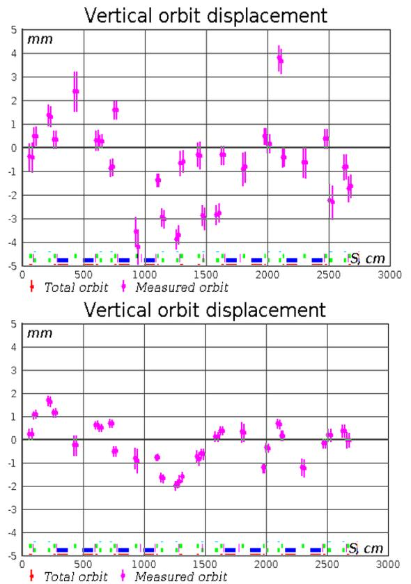
Figure 9: Closed orbit correction. Top – before correction, bottom – after.
