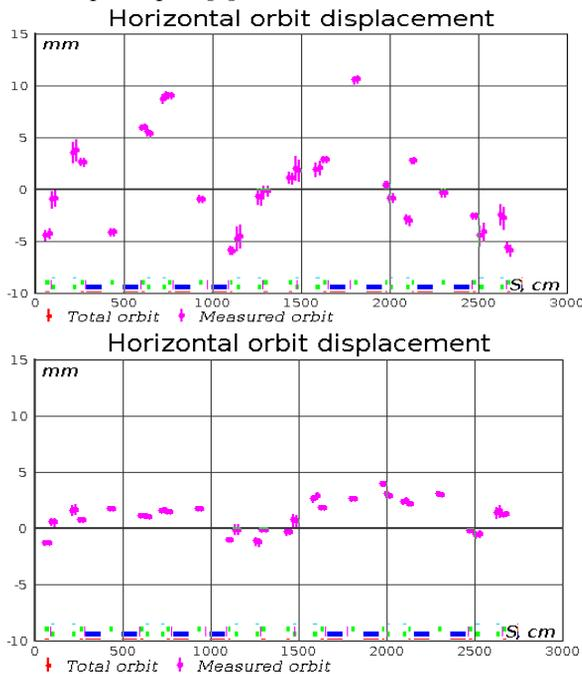
Figure 8. Closed orbit correction. Top – before correction, bottom – after.
