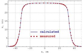
Figure 11: Field longitudinal distribution B<sub>y</sub>(s) at 9.9 kA.
