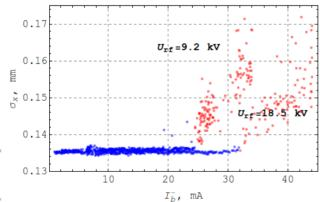
Figure 5: Horizontal beam size on 4M1L CCD (in place with non zero dispersion) as a function of beam current @ E=480 MeV.
