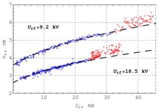
Figure 6: Bunch length as a function of beam current @ E=480 MeV.
