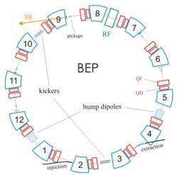
Figure 10: Booster synchrotron BEP layout.
