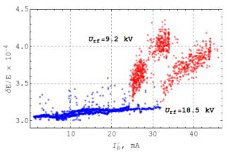
Figure 7: Beam energy spread as a function of beam current @ E=480 MeV.
