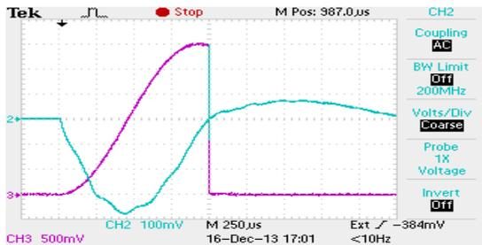
Figure 3: Prototyping measurement results. Voltage (10 kV/div) at the equivalent capacitance and input current (40 A/div) of the transformer.
