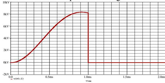
Figure 2: Shape of the voltage pulse on the plate simulated with PSPICE.
