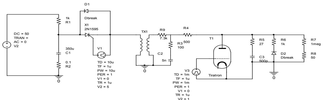
Figure1: PSPICE model of the power supply circuit.
