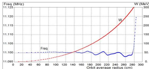
Figure 7: Orbital frequency  $Freq$  and energy of central proton  $W$  in isochronous field versus orbit average radius.
