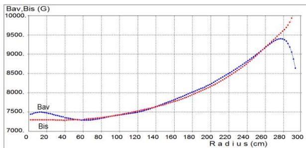
Figure 4: Average magnetic field  $B_{av}$  and isochronous one  $B_{is}$  versus radius.
