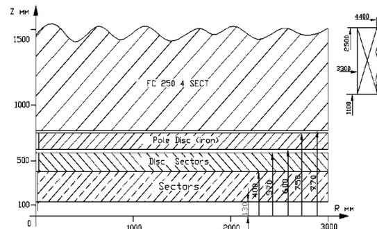
Figure 2: Scheme of the main elements location on vertical cross section.
