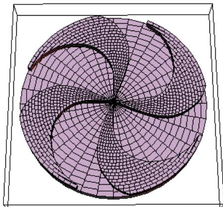
Figure 3: Configuration of the magnetic sectors.
