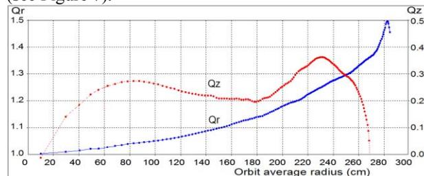
Figure 6: Frequencies of axial  $Q_z$  and radial  $Q_r$  oscillations versus orbit average radius.
