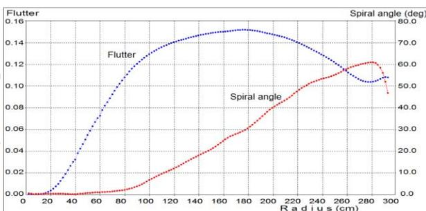
Figure 5: Flutter and spiral angle of the field versus radius
