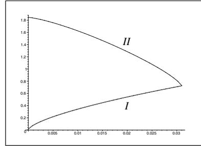
Figure 6: Dependence of the ion speed and temperature from coordinate.
