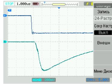
Figure 5: Pulse from photomultiplier tube.
