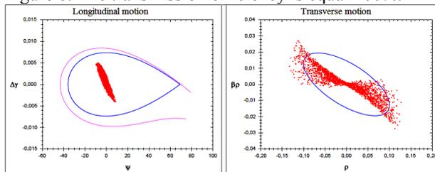
Figure 6: Longitudinal and transverse phase spaces in the fourth part with energy 214 MeV after phase variation.
