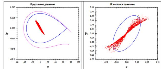
Figure 7: Longitudinal and transverse phase spaces in the fourth part with energy 200 MeV after phase variation.
