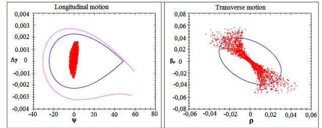
Figure 3: Longitudinal and transverse phase spaces in the fourth part with energy 200 MeV.
