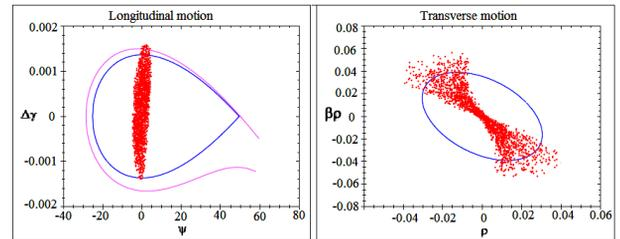
Figure 4: Longitudinal and transverse phase spaces in the fourth part with energy 150 MeV.
