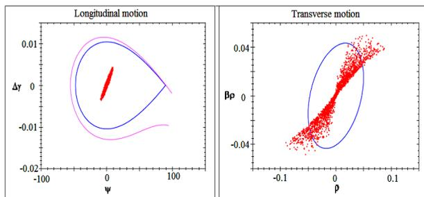
Figure 5: Longitudinal and transverse phase spaces in the fourth part with energy 200 MeV after phase variation.
