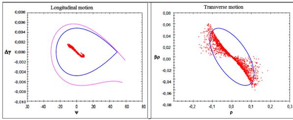
Figure 2: Longitudinal and transverse phase space in the fourth part.
