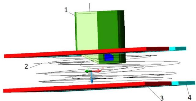
Figure 4: Central region structure: 1 – inflector RF shield, 2 – particle trajectory, 3 – dee, 4 – dummy dee.
