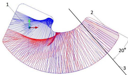
Figure 1: Spiral inflector cut: 1 – inflector entrance, 2 – inflector exit, 3 – cutting plane.
