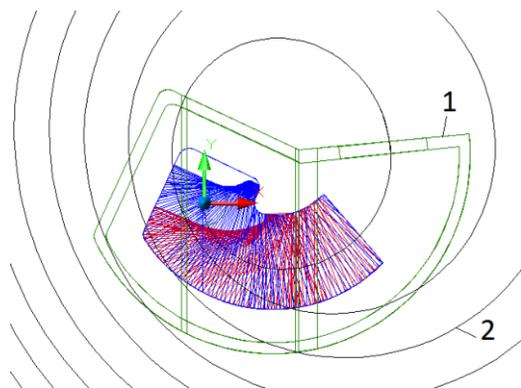
Figure 3: Particle trajectory in the central region: 1 – inflector RF shield, 2 – particle trajectory, 3 – dee, 4 – dummy dee.
