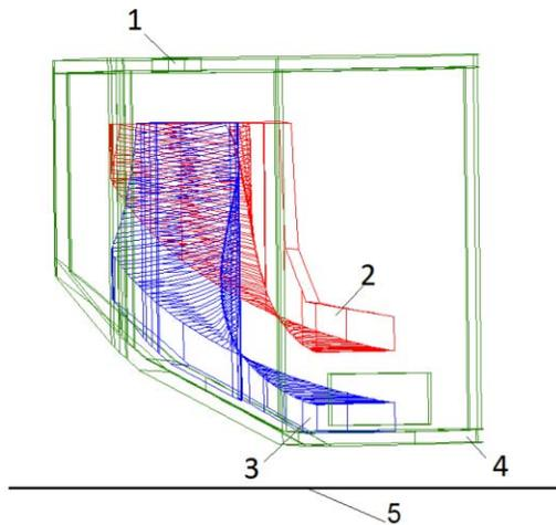
Figure 2: Inflector structure: 1 – inflector entrance, 2 – upper electrode, 3 – lower electrode, 4 – inflector RF shield, 5 – median plane.
