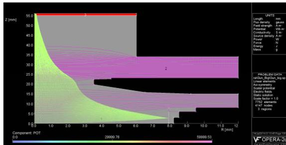
Figure 10: Electric field equipotential lines and electron trajectories for model with modified geometry.
