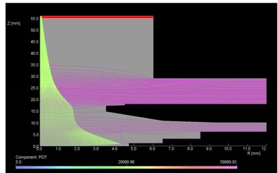
Figure 6: Electric field equipotential lines and electron trajectories for model with decreased anode potential.
