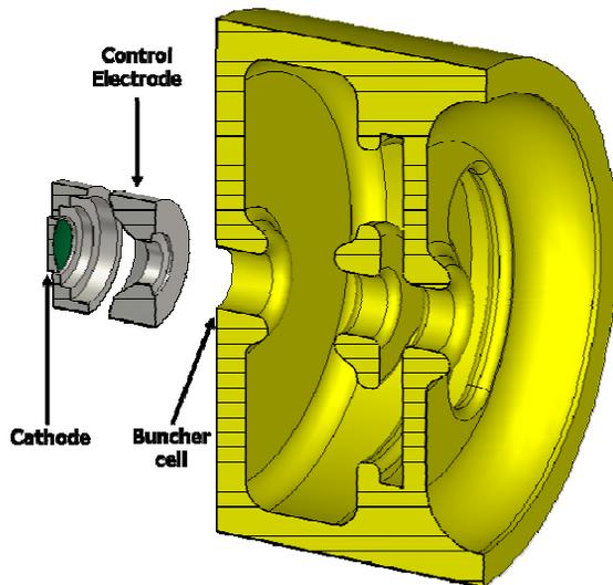
Figure 1: Cross-section of electron gun with buncher cell.
