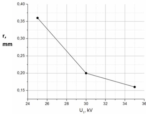
Figure 4: Beam radius over anode potential.
