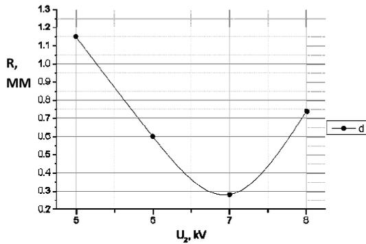
Figure 9: Beam crossover radius over control electrode potential plot.
