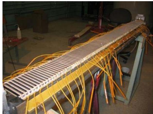
Figure 6: Assembling of 2 Tesla SC multipole wiggler for ALBA-CELLS (Spain).
