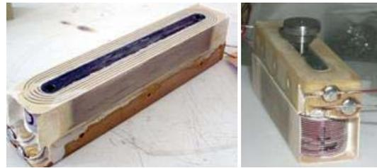
Figure 5: Main element of the medium field SC wigglers.
