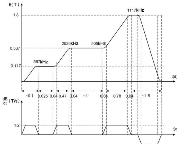
Figure 1: Booster magnetic field and acceleration frequencies.
