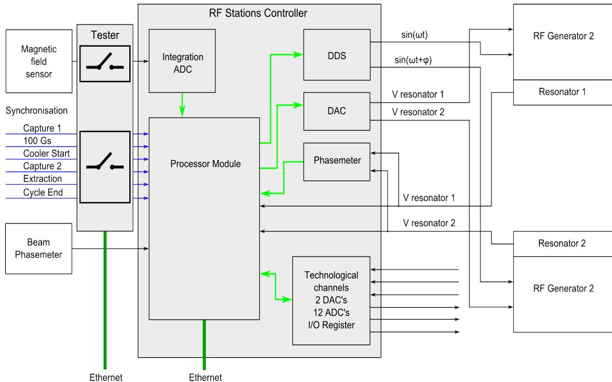
Figure 2: Control architecture.
