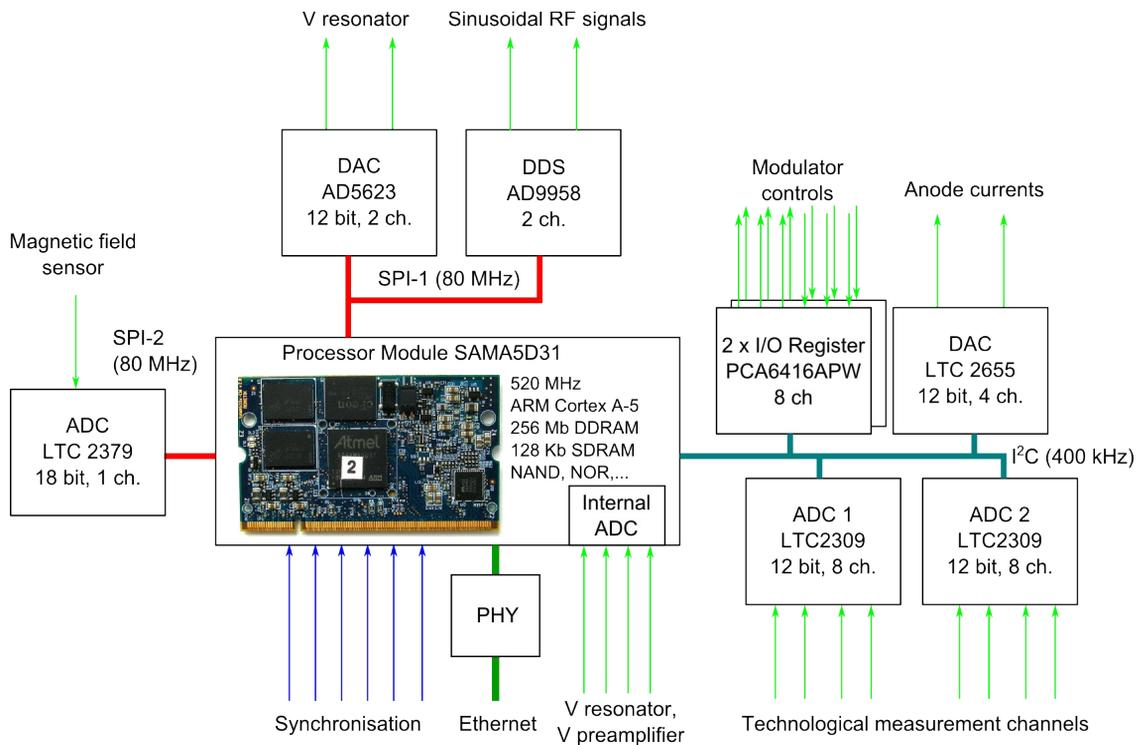
Figure 3: Controller module structure.
