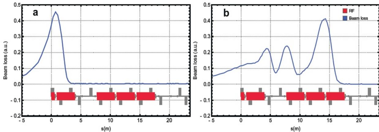
Figure 3: Beam losses: a) beam was dumped at the end of the 1st RF-structure, 20 m fiber was used; b) at the end of the 4th RF-structure, 60 m fiber was used.
