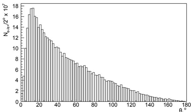
Figure 2: Angular distribution of secondary  $e^-/e^+$  relative to beam direction passing through optical fiber. 270 MeV electron beam with  $10^{10}$  electrons hits 2 mm steel vacuum pipe with  $1^\circ$  incident angle. Fiber is placed at the loss point. Total number of charged particles is  $0.5 \cdot 10^{10}$ .
