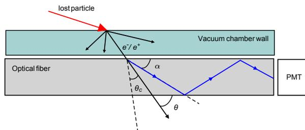
Figure 1: Scheme of beam loss monitor.
