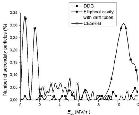
Figure 1: The number of particles percentage increase in the structure as a function of the field gradient for three resonator geometries smooth, fluted beam pipe and demountable damped structure.
