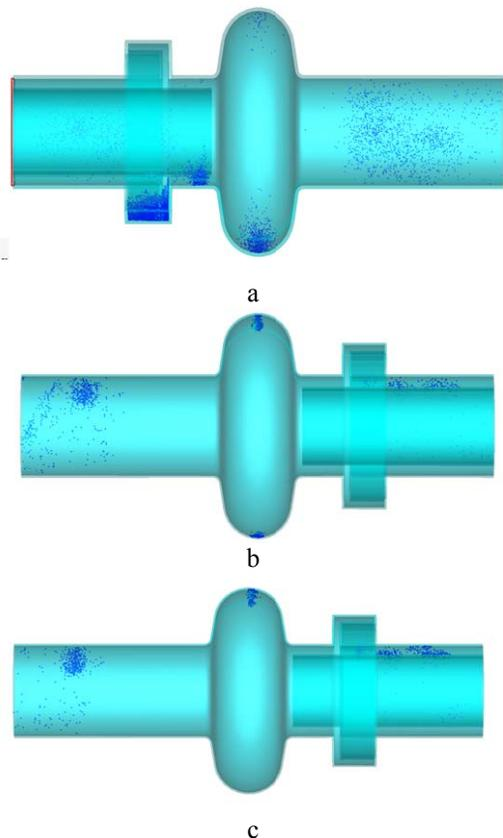
Figure 6: Regions of secondary electrons that remain active after 40 RF cycles. a) at 0.4 MV/m; b) at 7.5 MV/m; c) at 15 MV/m.
