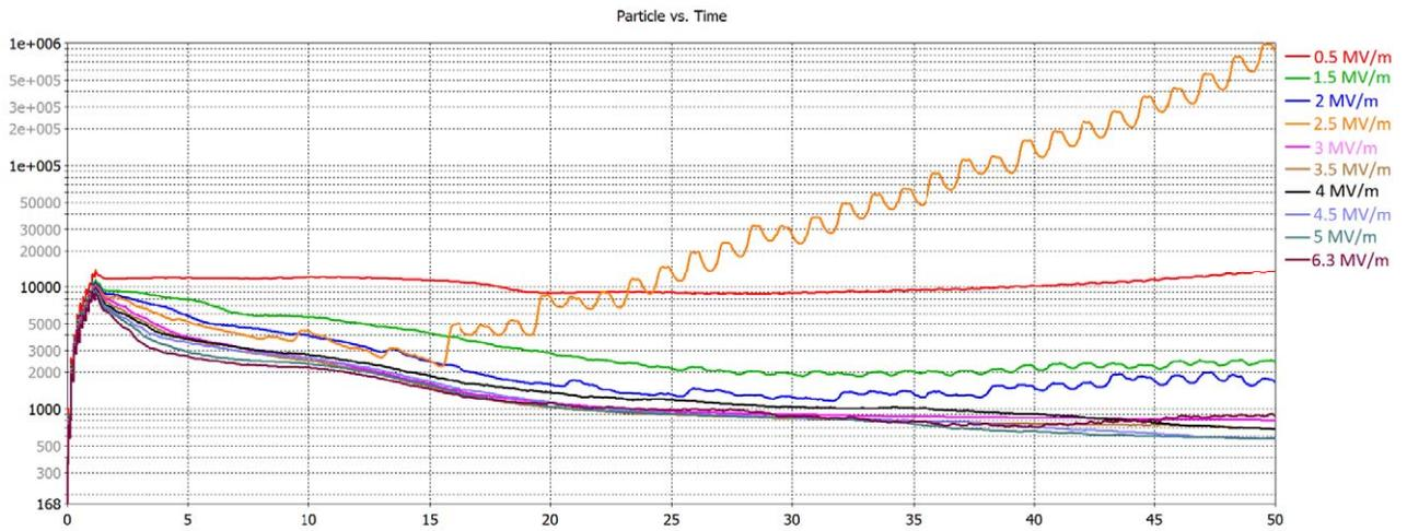
Figure 4: Number of particles increase in the structure as a function of time and different field gradients for demountable damped structure.
