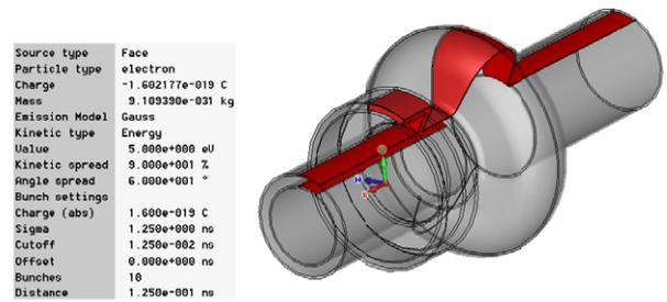
Figure 2: Demountable damped cavity (DDC).
