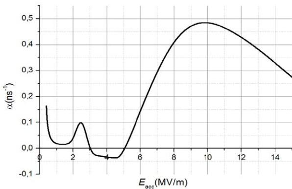
Figure 5: Avalanche growth rate at different levels of the accelerating gradient in demountable damped structure.
