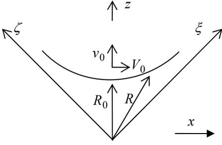
Figure 2: Particle motion in quadrupole magnetic field.
