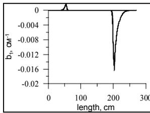
Figure 10: Quadrupole  $b_1(r,s)$  component of magnetic field of TM50 magnet. Orbits 2,4
