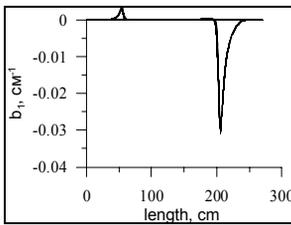
Figure 9: Quadrupole  $b_1(r,s)$  component of magnetic field of TM50 magnet. Orbits 1,5
