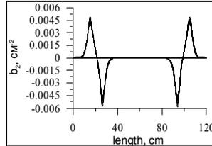
Figure 8: Sextupole  $b_2(r,s)$  component of magnetic field of IM90 magnet
