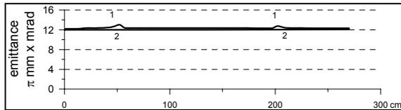
Figure 19: Horizontal (1) and vertical (2) beam emittances at orbits 2,4
