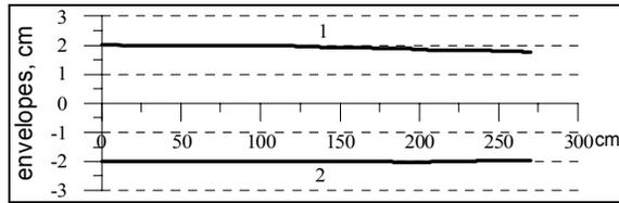
Figure 17: Horizontal (1) and vertical (2) beam envelopes at orbits 2,4
