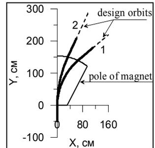
Figure 3: Reference orbits of TM50 magnet
