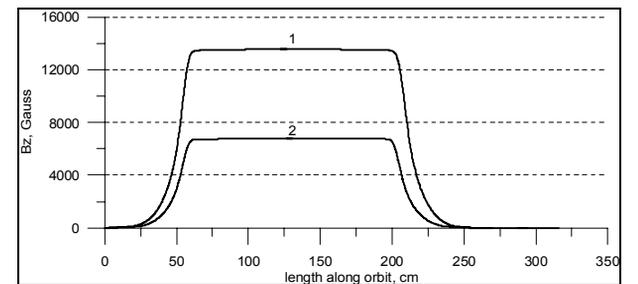
Figure 6: Bz field along reference orbits of TM50 magnet
