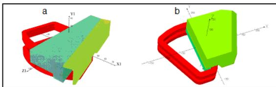
Figure 1: 3D models of IM90 (a) and TM50 (b) magnets
