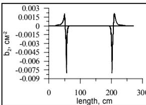
Figure 11: Sextupole  $b_2(r,s)$  component of magnetic field of TM50 magnet. Orbits 1,5
