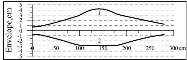
Figure 13: Envelopes of the ion beam for horizontal (1) and vertical (2) motion
