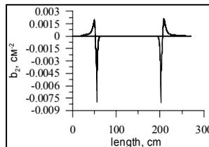
Figure 12: Sextupole  $b_2(r,s)$  component of magnetic field of TM50 magnet. Orbits 2,4
