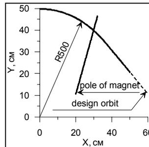
Figure 2: Reference orbit of IM90 magnet
