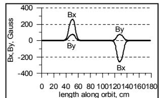
Figure 5: Bx,y field at 2 cm higher reference orbit of IM90 magnet
