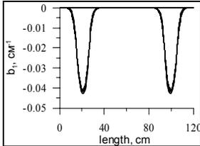
Figure 7: Quadrupole  $b_1(r,s)$  component of magnetic field of IM90 magnet
