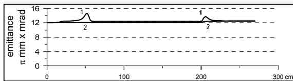
Figure 18: Horizontal (1) and vertical (2) beam emittances at orbits 1,5
