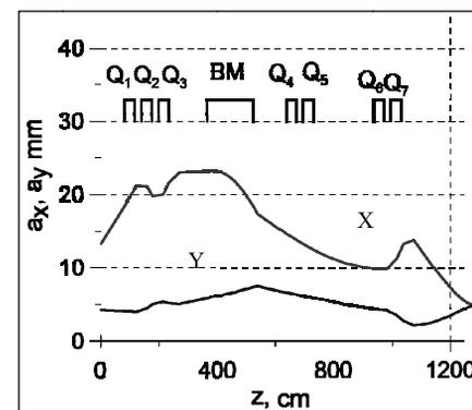
Figure 4. Transportation of  $^{238}\text{U}^{43+}$  ions in beam line 2.
