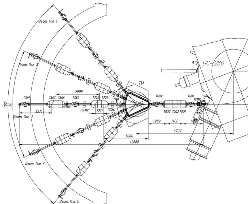
Figure 1: Lay-out of the beam lines for heavy ion transportation.
