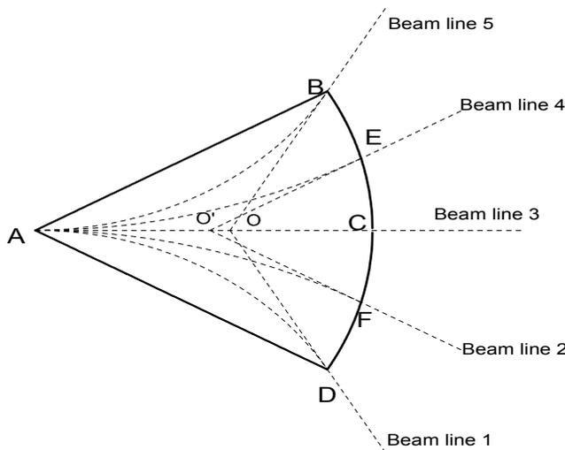
Figure 2. Scheme of TM bending magnet.
