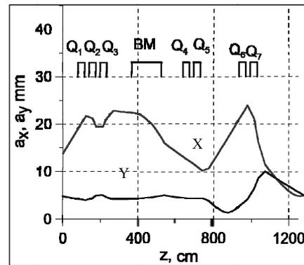
Figure 3. Transportation of  $^{48}\text{Ca}^{9+}$  ions in beam line 1.
