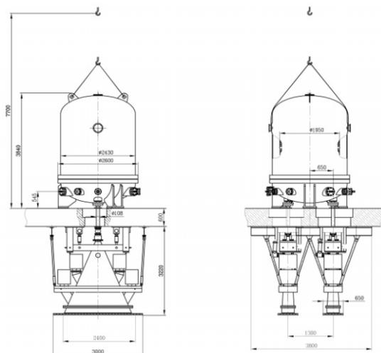
Figure1: General view and main parameters of the «Electron-23» accelerator.
