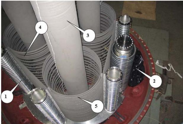
Figure 2: Support columns (1), AT with electromagnetic screens (2), magnetic cores of the HV rectifier primary winding phases (3), gradient rings (4) and electromagnetic screens (5).
