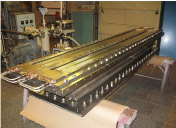
Figure 3: Beam extraction device of the «Electron-23» accelerator at a test facility in NIIEFA.
