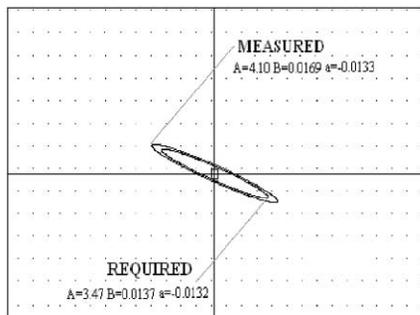
Figure 3: Root-mean-square ellipses of the transversal phase volume of the beam at the RFQ input (grid: 0.98 mm by 43.61 mrad).
