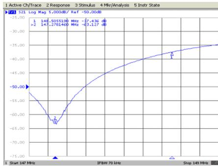
Figure 6: Frequency response characteristic before tuning.
