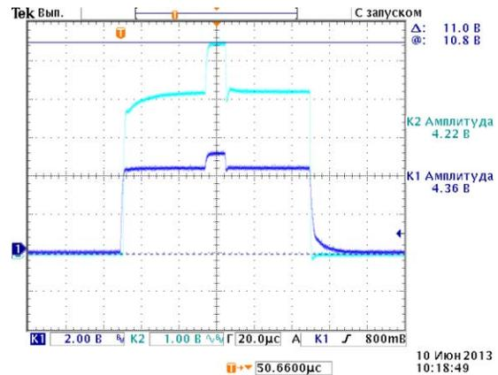
Figure 8: Oscillograms of the power amplifier: output RF impulse (up) and generator impulse (down).
