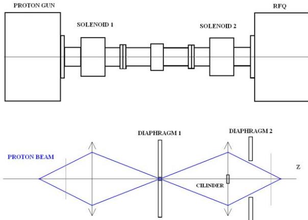
Figure 2: Optic scheme of the matching channel.
