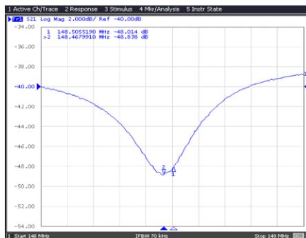
Figure 7: Frequency response characteristic after tuning.
