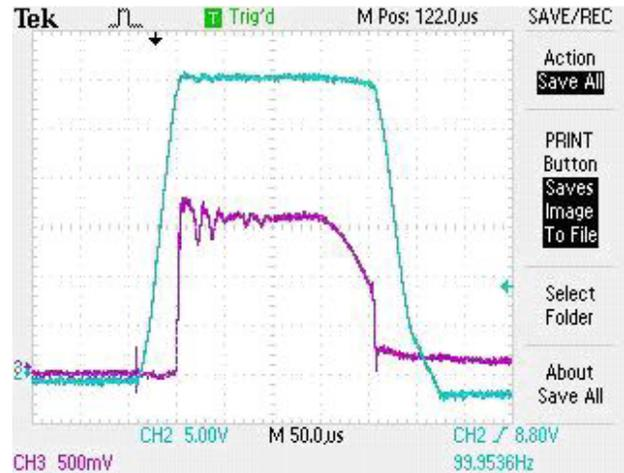
Figure 1: Oscillogram of the HVPG pulse at 100 Hz PRR (the pulse with smaller amplitude is the top of the HV pulse on a larger scale).
