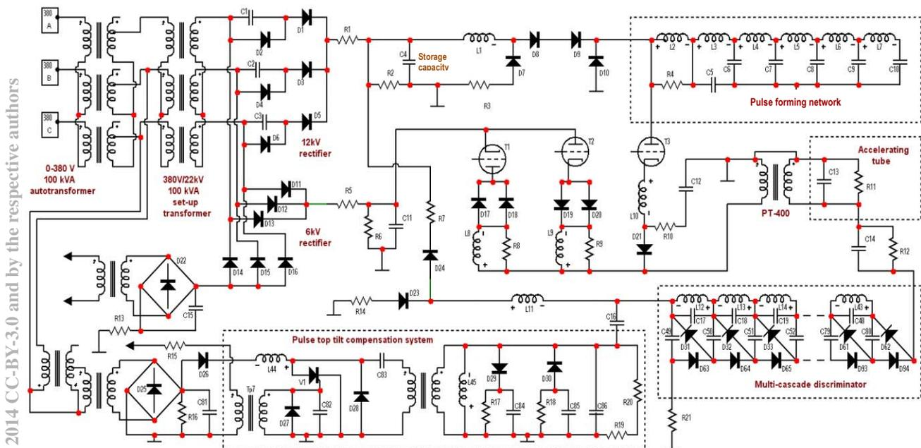
Figure 2: The proton injector HVPG electrical circuit.
