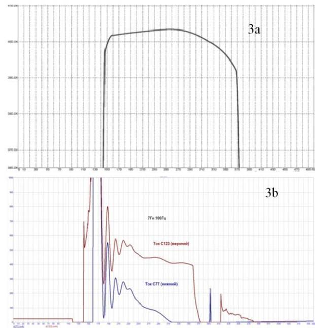
Figure 3: Simulation results for HV pulse top (3a) and for "upper" and "lower" MD capacitors current shape (3b, upper and lower curve, respectively).
