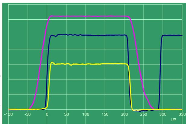
Figure 5: Oscillograms of the HVPG pulse at 100 Hz PRR (the yellow pulse with smaller amplitude is the top of HV pulse on a larger scale). Also there are (dark blue) the beam current curve and 100 mA calibrator pulse (on the right).
