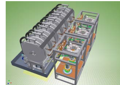
h=2 acceleration cavity for faster ramping
