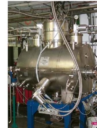
Fig. 2-4 Photo of 7 Tesla WLS inserted into BESSY-2 straight section.
